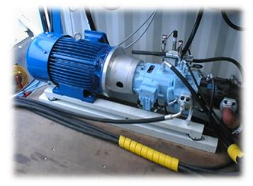
In case of 24Vdc supply failure, The hydraulic pump can be maneuvered manually.
